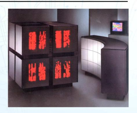
A "massively parallel" hypercubic arrangement of **32k single bit processors**
